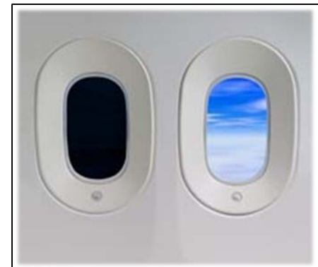
Boeing 787 passenger windows measure approximately 12" wide by 18" long
