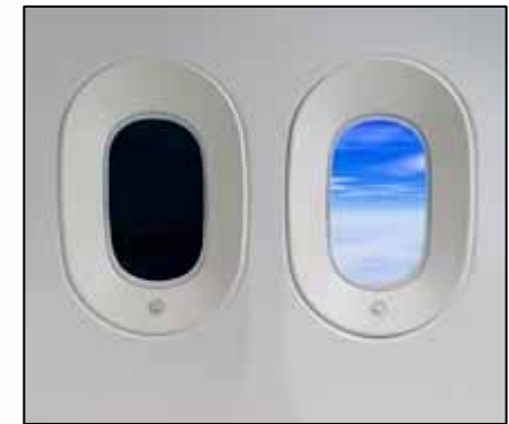
Passenger windows measure approximately 12" wide by 18" long
