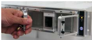
Pluggable canisters are easy to insert and remove.
